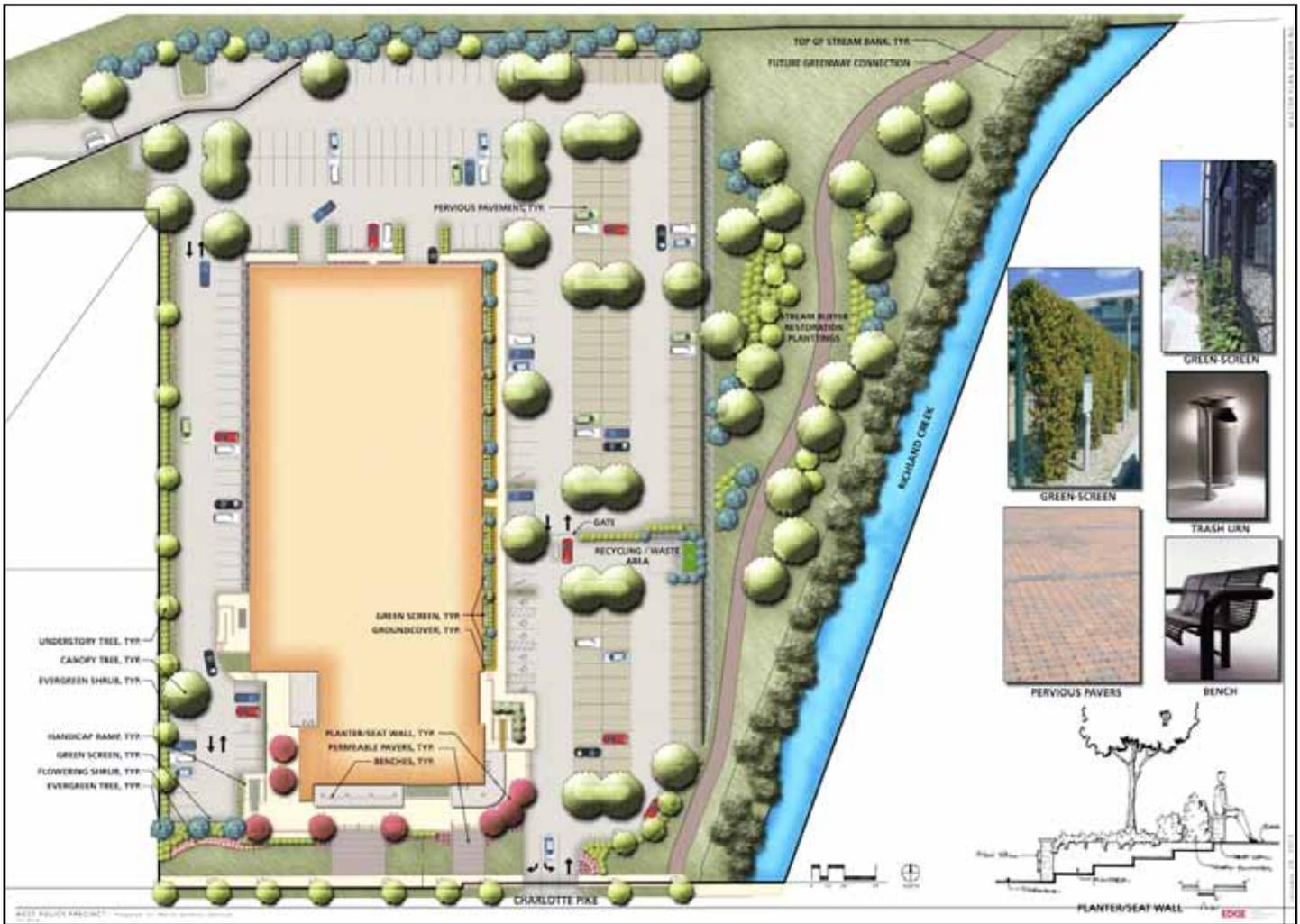
Drawing of Revised W. Precinct Plan. Dark gray parking is pervious pavement and will filter-out pollutants
